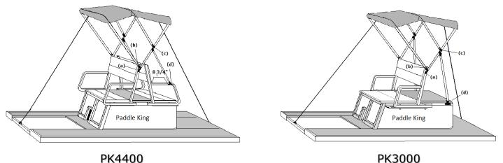
1. Remove canopy from boat by unhooking front and rear straps and removing thumb screws.
